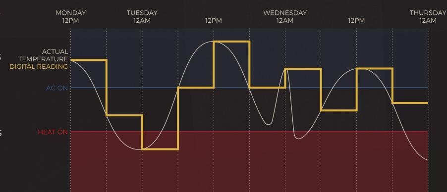
IN THIS EXAMPLE, the sensor is taking heat readings every six hours. We see that while the digital readings generally follow the curve of the actual temperature, it doesn't always get it quite right and sometimes misses important details, like the unexpected spike in heat on
