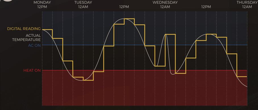
HERE WE'VE TAKEN THE SAME TEMPERATURE DATA, but doubled the sample rate of the digital sensor, resulting in much more accurate heating and cooling and hopefully, a more
